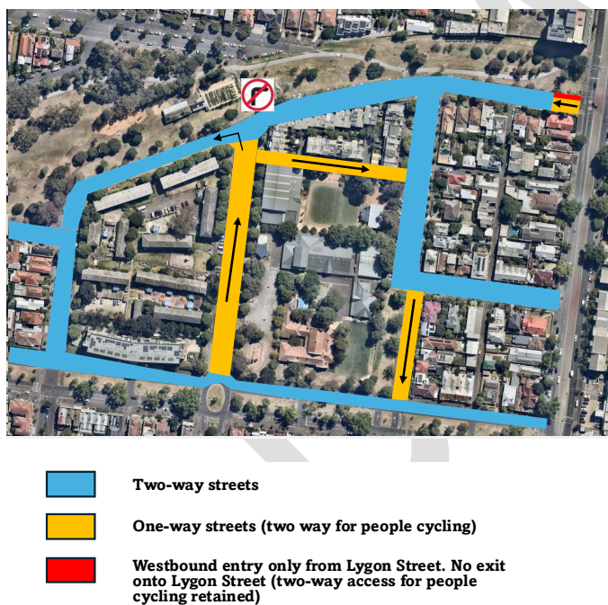
Figure 4-10: Design Option 3 Traffic Movement Summary
