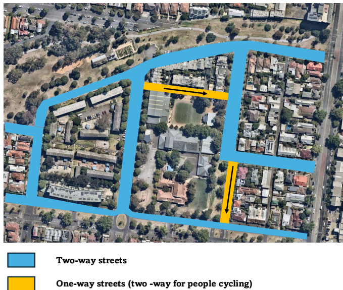
Figure 4-8: Design Option 1 Traffic Movement Summary
